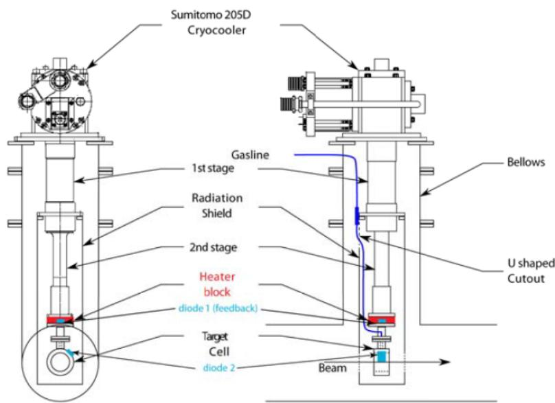
Figure 9: A diagram of the Liquid Deuterium Target illustrating how it will sit in the beam-pipe.
