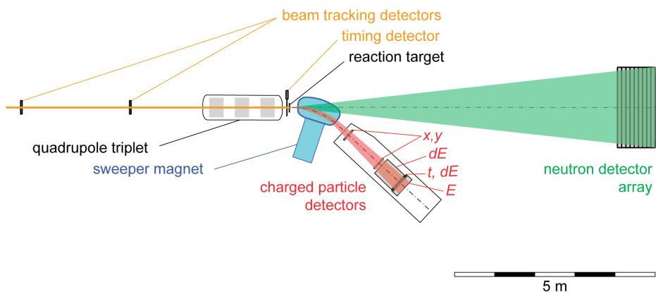
Figure 6: Schematic layout of the Sweeper–MoNA setup.
