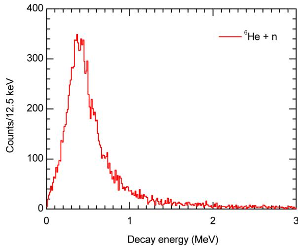
*Figure 2:* The reconstructed decay-energy spectrum for the neutron-unbound ground state in  ${}^7\text{He}$ , which is unbound by 450 keV and which has a width of 160 keV. The data were taken during the commissioning of the Sweeper Magnet and the MoNA neutron detector at NSCL.
