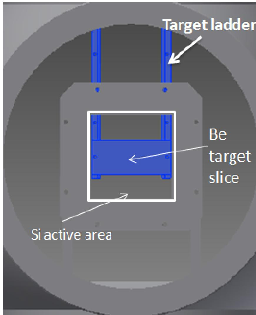
Figure 8: Beam eye-view of the proposed Si-Be segmented target to be used at NSCL.
